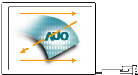
Fig. 1 Normal scan (Pin4, DPS = Low or NC)
