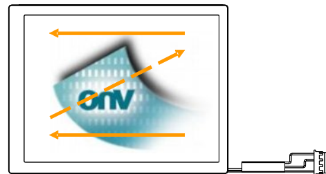
Fig. 2 Reverse scan (Pin4, DPS = High)
