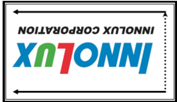
RPF1 = high: display with 180degree rotation
