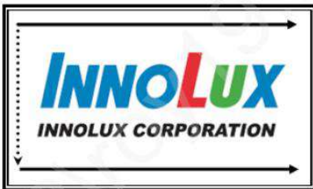
Fig. 1 Normal scan (PCBA on the bottom side) ( pin 17, REV_SCAN = Low )
