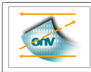
Fig. 2 Reverse scan (Pin19, RSV = High or VDD)
